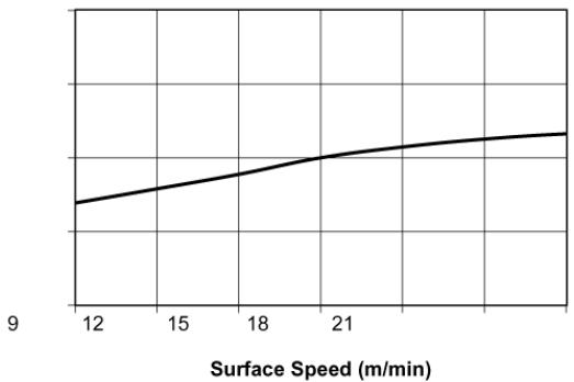
Graph 1: Coefficient of friction of G300® as a result of the running speed;  $p = 7.6 \text{ kgf/cm}^2$
